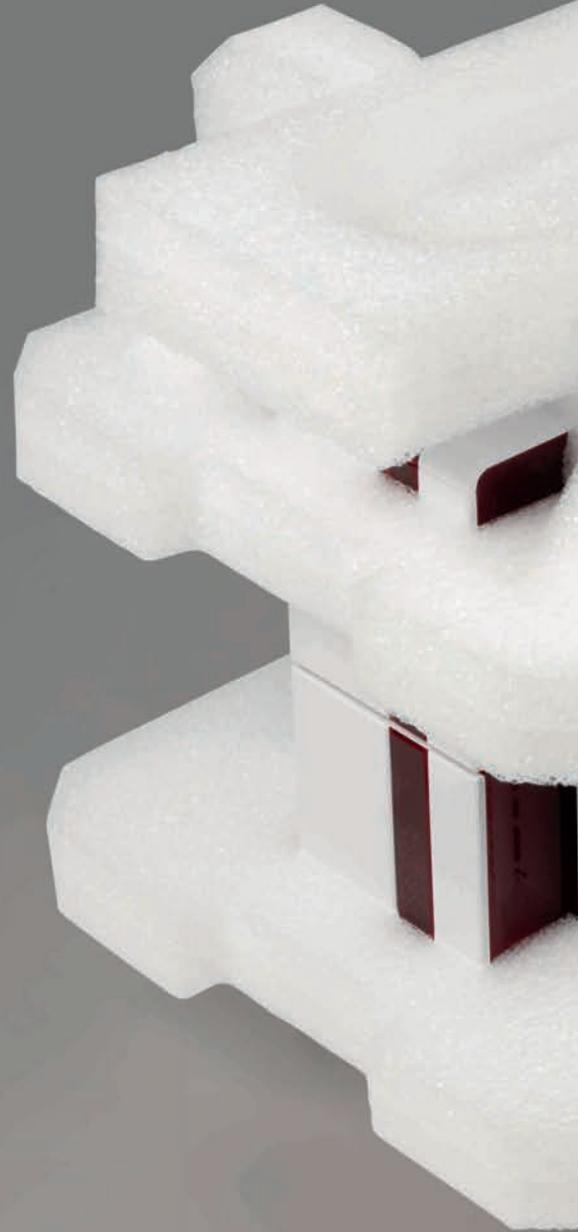
We process foam by waterjet cutting, punching, contour cutting, milling and other manufacturing processes to make tailored, volume-optimized, secure transport packaging for sensitive goods. We produce excellent foam packaging made of polyethylene foam (PE foam), polyurethane foam (PU foam) or polystyrene foam (PS foam) or Styrofoam®, which optimally protects packaged goods against impacts, vibration, friction, scratches and electrostatic charges (ESD protection).
